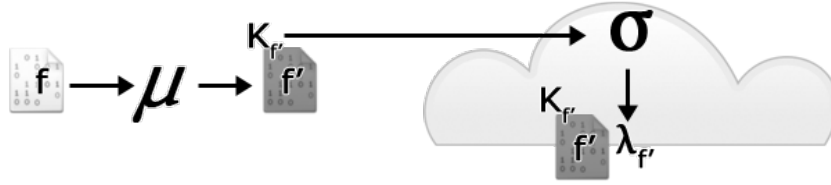
Fig. 2. A visualisation of the notation used to describe the linkability attack. The figure shows how a file is mapped into its internal representation in the storage service by the mapping \mu , and then its storage location is determined by the function \sigma .
