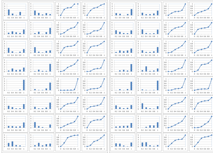
Fig. 6. Spatial array of heavy fluid concentrations at t = 50 , for z in the midplane, as PDFs (bar graphs) and as CDFs (line graphs), Left: Medium grid. Right: Fine Grid.
