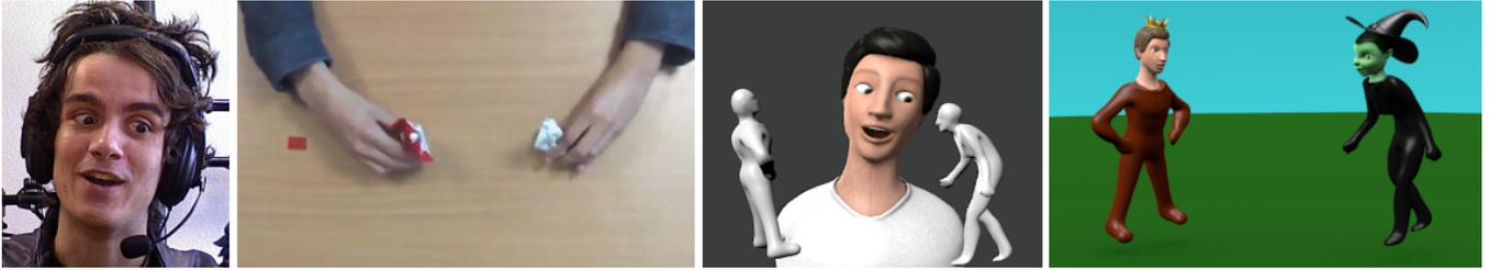
**Figure 3:** Corresponding frame for: (a) the front Kinect video data displaying the storyteller's expressions, (b) the top Kinect video data with the current orientations and positions of the figurines, (c) a reconstructed scene including a virtual storyteller with directly transferred expressions and virtual figurines with directly transferred movements and (d) the final animated version of the story.
