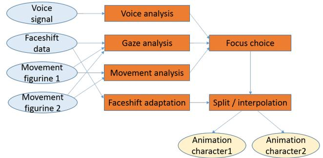
**Figure 2:** System workflow: the voice signal, motion recorded with FaceShift and figurine movements are analyzed in order to determine the focus turns of the characters to which the adapted motion is transferred. Next, the separate animation data for the two characters is obtained by splitting the storyteller's recorded data and interpolating the missing motion from the non-focused parts.
