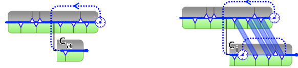
Figure 5. Left: applying a command C_a to a past state always generates a new state of history regardless of its existing ‘children’ . Right: inserting a command C_i in an existing sequence of commands generates a new subtree, with replicated commands from the original branch (blue halo). The user travels to the end of the branch to see the effect of the insertion.
