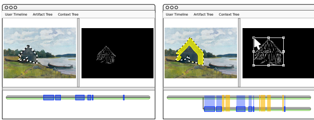
Figure 11. Left: displaying the stroke shapes corresponding to the selected ‘paint’ commands (right panel). Right: scaling these strokes generates a parallel branch (bottom panel) and raises paradoxes (in yellow) with later, intersecting ‘paint’ commands.
