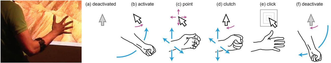
**Figure 1: Myo armband (left) and Myopoint interaction (right): (a) initially deactivated; (b) activate by raising clenched fist and releasing; (c) point by moving arm with relaxed hand; (d) clutch with clenched fist; (e) click by spreading all fingers; (f) deactivate by lowering clenched fist and releasing.**
