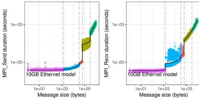
Figure 1. Communication time between two nodes of the Taurus cluster (Ethernet network). The duration of the communication with either MPI\_Send or MPI\_Recv are modeled as piece-wise linear functions of the message size.
