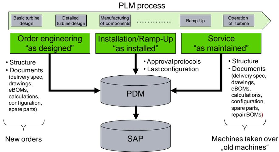
Fig. 3. Framework for the new PLM Process Concept
