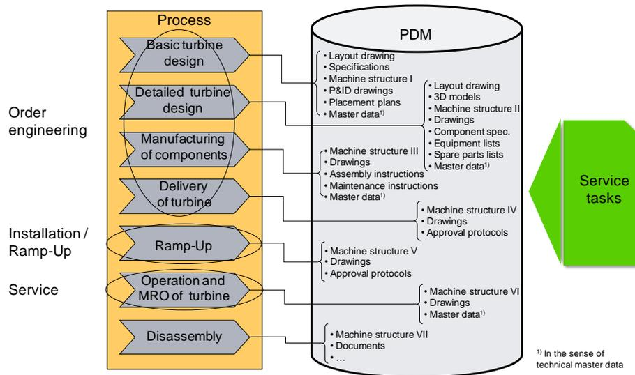
Fig. 4. Engineering Data generated throughout the Steam Turbine Lifecycle and PLM Process
