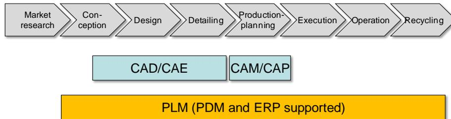
**Fig. 1.** Simplified Product Lifecycle of a Steam Turbine
