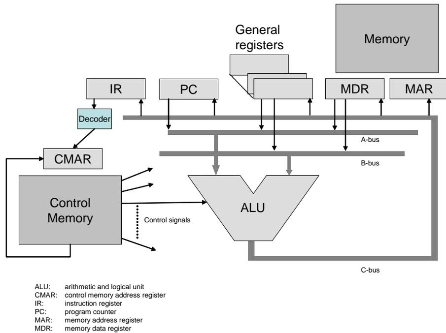
By placing an extra register at the entrance of the ALU one can delete one bus and by adding a further extra register at the second entrance even one bus suffices. It will be clear that the speed of instruction execution in that case proportionally decreases.
