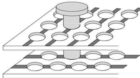
**Figure 4:** Schematic detail of a matrix board
