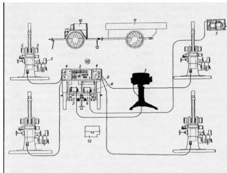
Figure 3.2: The GAMMA-Juhász anti-aircraft gun-director controlled 4 guns simultaneously
