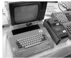
Figure 13.3: The ABC 80 and the BRG Tape recorder
