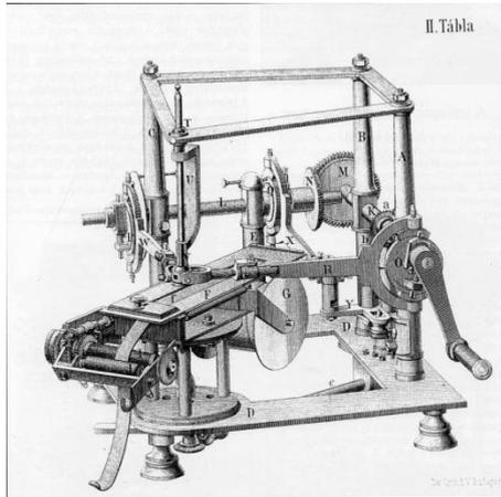
Figure 2.4: Mechanical graphical analog calculator
