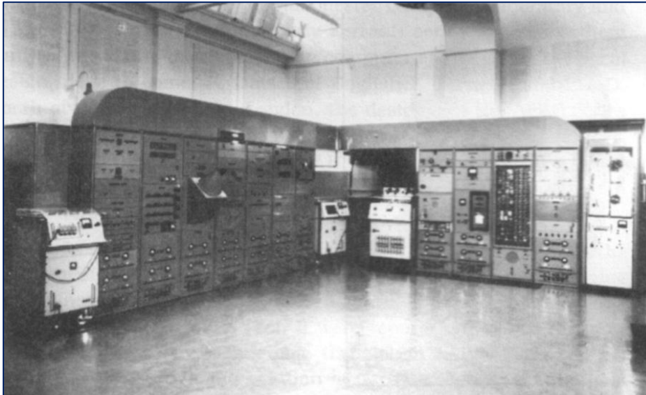
The Elliott 403's Input Converters: Rocket Telemetry Converter (left) and Doppler Radar Converter (right) – from T. Pearcey 'A History of Australian Computing' – Chisholm Institute of Technology 1988)
