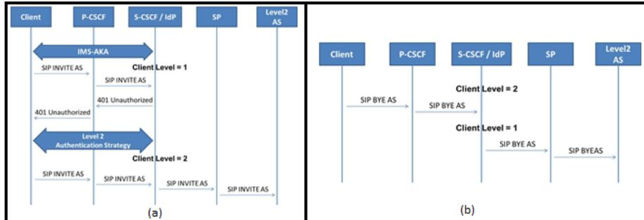
**Fig. 4.** (a) Client wanting to access a level 2 application server message flow.
