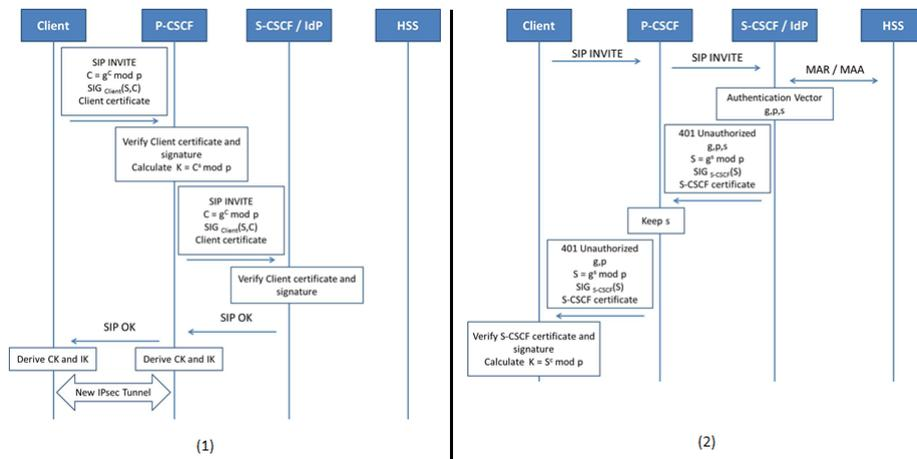
Fig. 5. Authenticated Diffie-Hellman using digital signature for IMS
