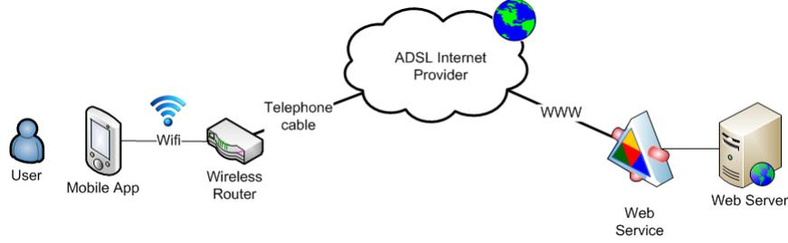
**Fig. 3.** Wi-Fi / ADSL based Transfer Architecture
