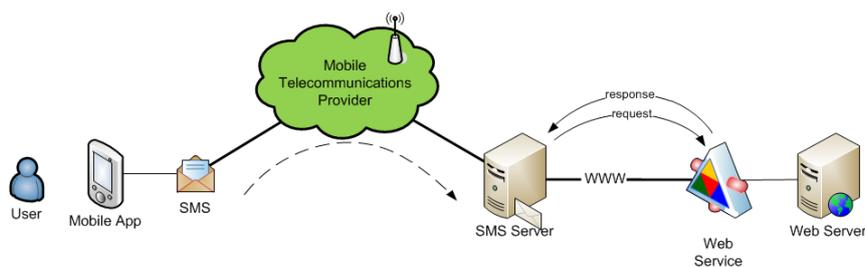
**Fig. 1.** SMS based Transfer Architecture
