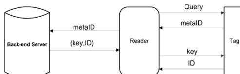
**Fig. 1.** Hash-Locking: A reader unlocks a hash-locked tag
