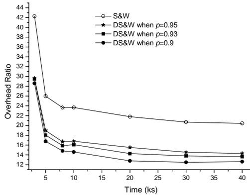
**Fig. 1.** Overhead ratio comparison between DS&W and S&W
