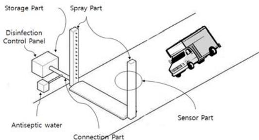
**Fig. 3.** Automatic Vehicles Disinfection System
