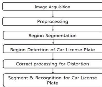
**Fig. 4.** Algorithm for Vehicles Recognition
