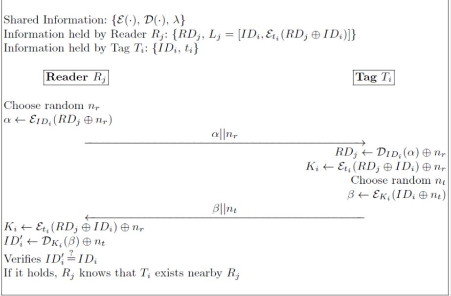
Fig. 1. Chun et al.'s RFID tag search protocol
