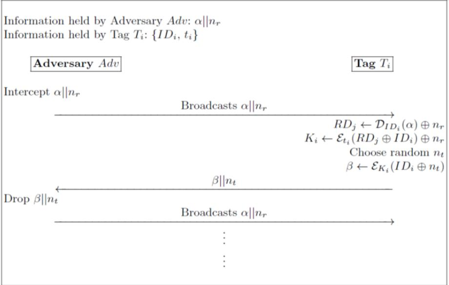
**Fig. 2.** DoS Attack against Chun et al.'s Protocol
