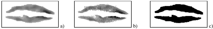
Fig. 1. Steps of lip area detection: a) the image after evaluating pixels against a threshold, b) after blurring, c) the detected lip area.
