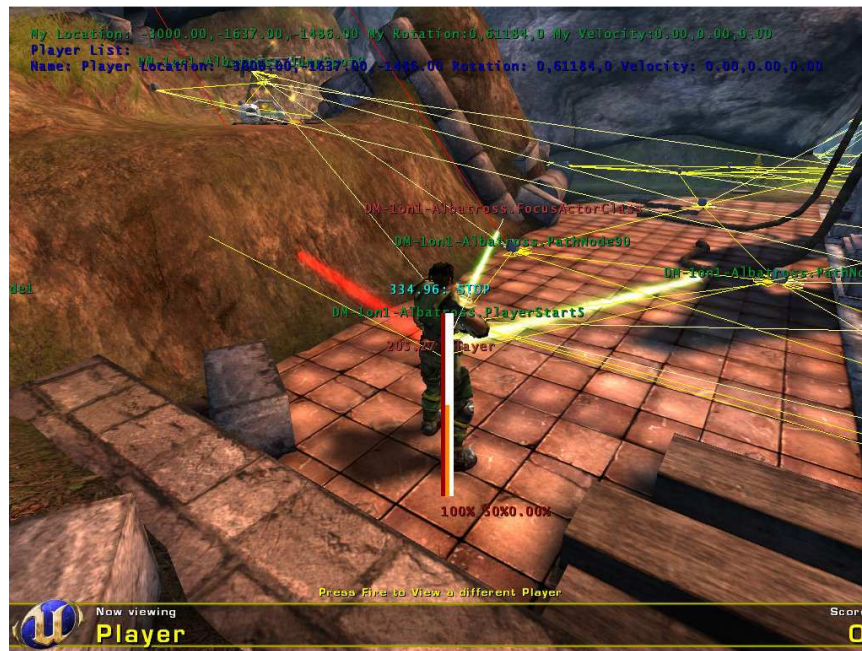
Fig. 1. Debugging features of Pogamut GB include navigation points and navigation grid visualization, raycasting visualization, bot health, armor and field of view visualization, general game information, etc. The screenshot is from UT 2004.
