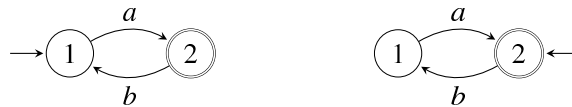
Fig. 8. SPA G (left) and DFA a \setminus G for the left quotient by the string a (right); projection P : \{a, b\}^* \rightarrow \{b\}^* .
