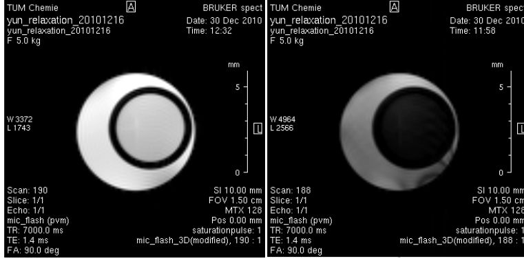
FIGURE 1. Experimental results: The inner circle shape sample mimics the deoxygenated blood, where T_1 = 1.3s and T_2 = 50ms ; the outside moon shape sample corresponds to the oxygenated blood, where T_1 = 1.3s and T_2 = 200ms . (left) Without control, (right) Optimized contrast.
