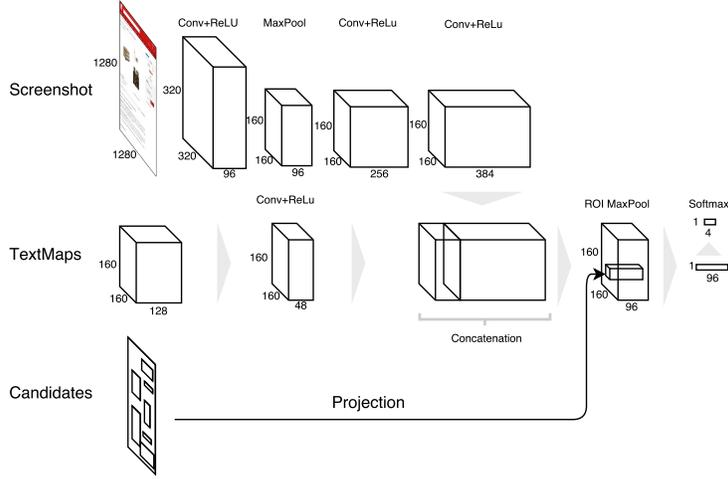
**Fig. 3.** Architecture of our CNN: Upper part represents visual feature extraction, which is then combined with textual features (middle). Coordinates of candidate boxes are projected to final feature tensor and resulting vector is extracted using ROI MaxPooling. Finally, linear model with softmax classifies vector into predefined classes.
