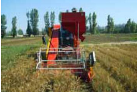
Fig. 4. Hanging harvester in China
