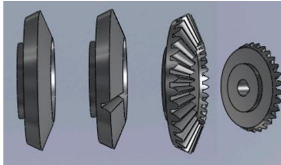
**Fig. 2.** Creating process of the bevel gear
