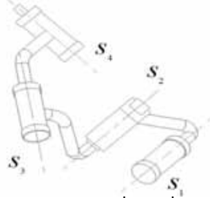
Fig. 7. Structur of Limb RPRR-1F1M( s_2 \perp s_{r1}, s_1 \perp s_{r2}, s_3 \perp s_{r2}, s_4 \perp s_{r2}, s_1, s_3, s_4 and s_{r2} are in the same plane )
