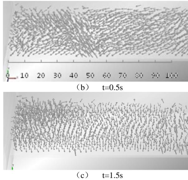
**Fig. 4.** Instantaneous velocity vector of seeds movement ( $f=50\text{HZ}$ )
