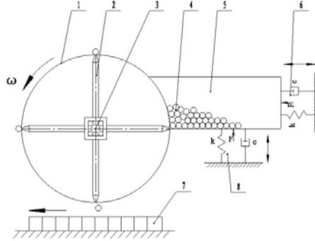
1.Cylinder 2.Permanent magnet 3.Drive shaft 4.Seed 5.seed box
