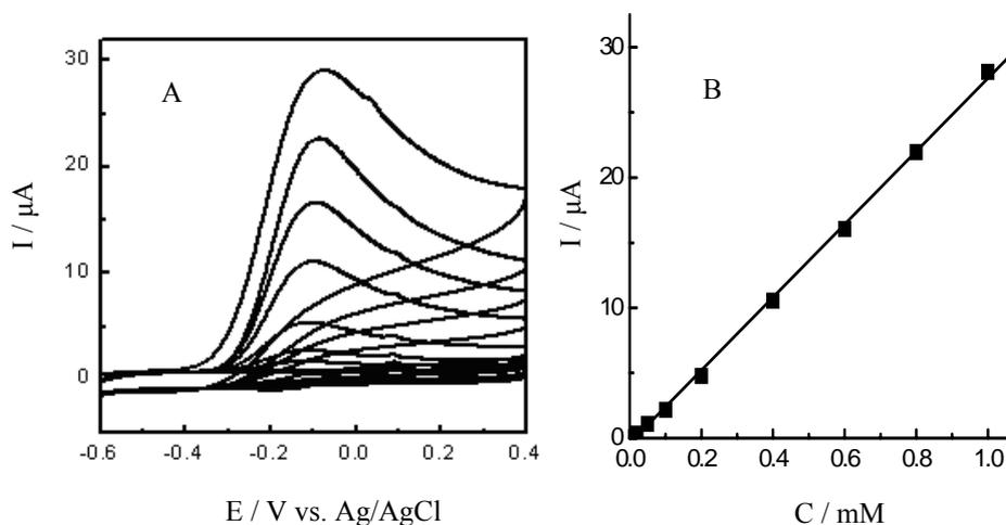
**Fig. 3.** (A) Typical CVs obtained at activated SPCE in 0.1 M phosphate buffer (pH 7.0) containing AA with different concentrations of 0.00, 0.01, 0.02, 0.05, 0.10, 0.20, 0.40, 0.60, 0.80 and 1.00 mM. Scan rate,  $100\text{ mV s}^{-1}$ . (B) Plot of current response vs the concentration of AA.
