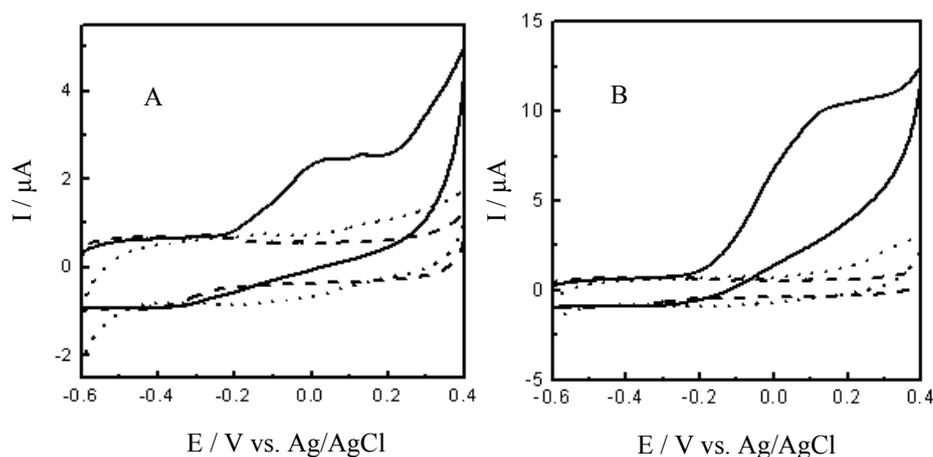
**Fig. 4.** CVs obtained at activated SPCEs in 0.1 M phosphate buffer (pH 7.0) in the absence (*dashed lines*) and presence (*solid lines*) of diluted cabbage sample (A) and orange sample (B). The dotted lines in (A) and (B) refer to the responses of the mixture of AAox and each diluted sample after 15min, respectively. Scan rate, 100  $\text{mV s}^{-1}$ .
