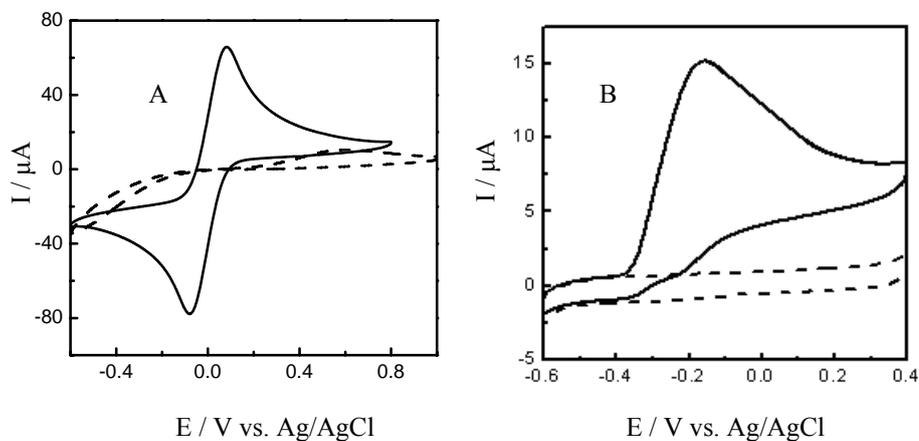
**Fig. 2.** (A) Typical cyclic voltammograms (CVs) at a fresh SPCE in 0.1 M phosphate buffer (pH 7.0) containing 5 mM  $K_3Fe(CN)_6$  before (*dashed line*) and after (*solid line*) electrochemical pretreatment. Scan rate,  $100\text{ mV s}^{-1}$ . (B) CVs obtained at a fresh SPCE in 0.1 M phosphate buffer (pH 7.0) in the absence (*dashed line*) and presence (*solid line*) of 0.50 mM AA after electrochemical pretreatment. Scan rate,  $100\text{ mV s}^{-1}$ .
