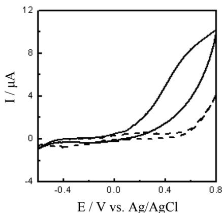
**Fig. 1.** CVs obtained at a fresh SPCE in 0.1 M phosphate buffer (pH 7.0) in the absence (*dashed line*) and presence (*solid line*) of 0.50 mM AA before electrochemical pretreatment. Scan rate, 100 mV s<sup>-1</sup>.
