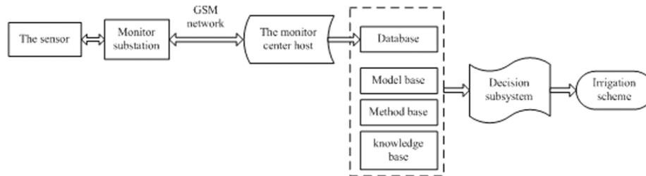
**Fig. 3. Work principle flowchart of intelligent decision subsystem**
