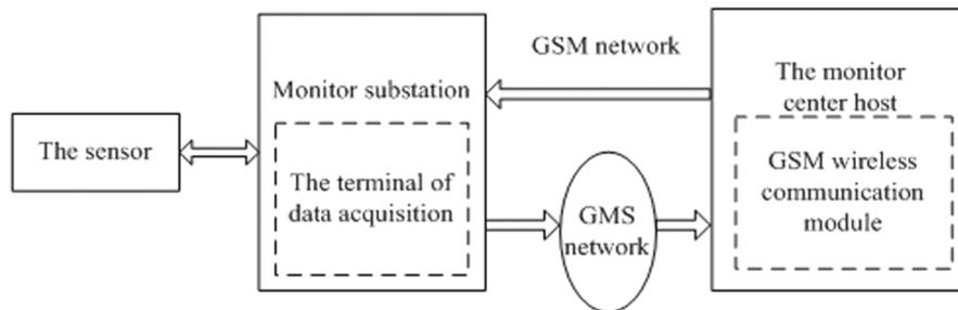
**Fig. 2. Work principle flowchart of data acquisition system**
