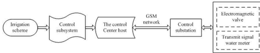
**Fig. 4. Work principle flowchart of automatic control subsystem**
