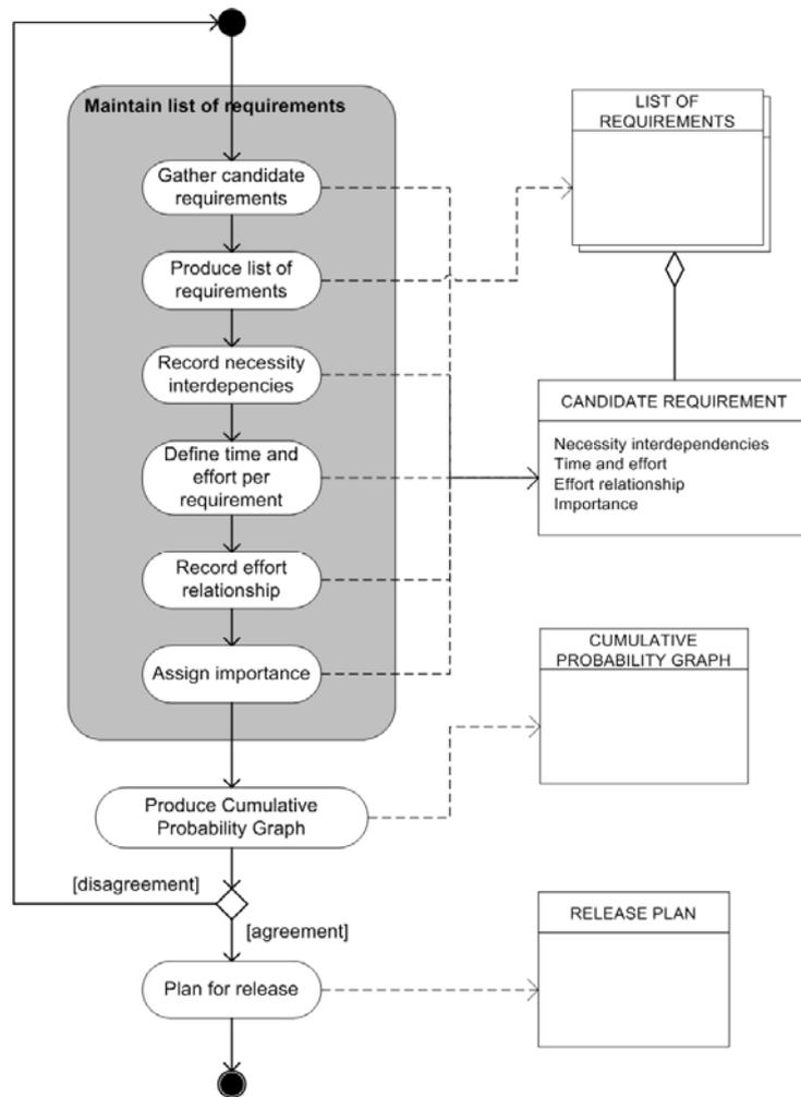
Fig. 2. PDD of the Requirements Triage method
