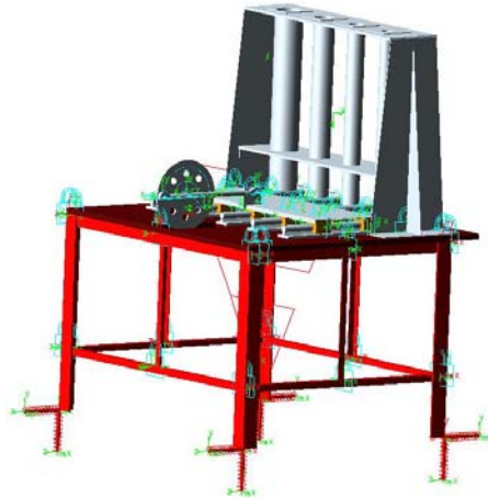
Fig. 1. Virtual prototyping of the lotus root slicing machine
