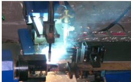
Fig.8. Automatic welding device in operation
