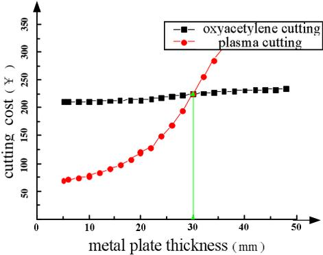
Fig.4. Cutting cost curve of plasma and oxyacetylene
