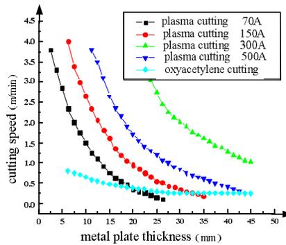
Fig.5. Cutting speed curve of plasma and oxyacetylene
