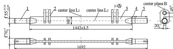
1 end axle; 2 pulling board; 3 brake beam body; 4 sleeve gasket working surface; 5 brake shoe working surface.
