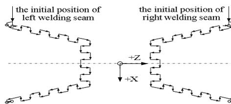
Fig.6. The welding path of new end axles
