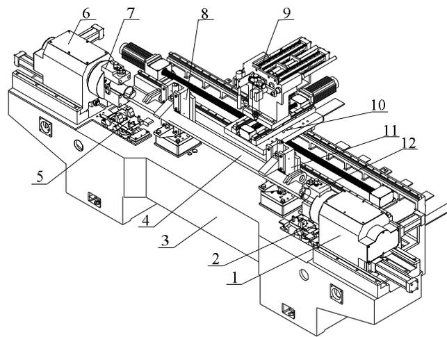
1,6 drive box; 2,5 bracket; 3 machine tool bed; 4 brake beam; 7,12 rotational device;
