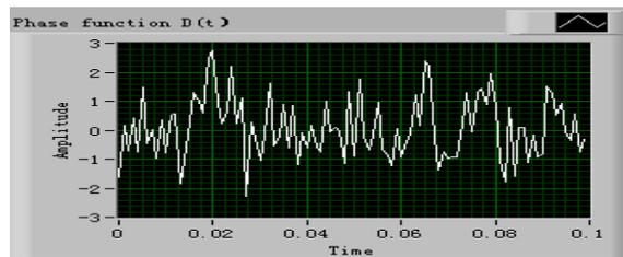
**Fig.7.** phase-shifts  $D(t)$  oscillogram when the amplitude is too large.
