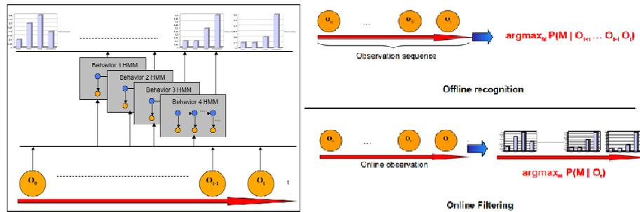
Fig. 5. Concurrent HMMs (left) Recognition Modes (right).
