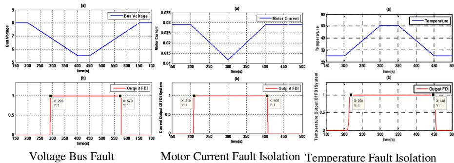
Fig.5. Three Fault Isolation and their sensitivity to changes of voltage, current, temperature
