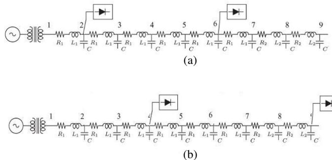
Fig. 4. Radial power distribution line: (a) Case I, (b) Case II.
