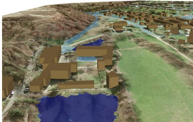
Figure 4. First results of the 1D-2D-hydrodynamic model DYNA-GeoCPM for the test-catchment area “Lüntenberg” in Wuppertal [15].
