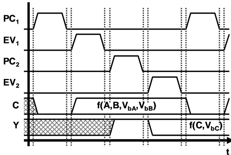
Fig. 4. Two-stage dynamic logic clock signal scheme
