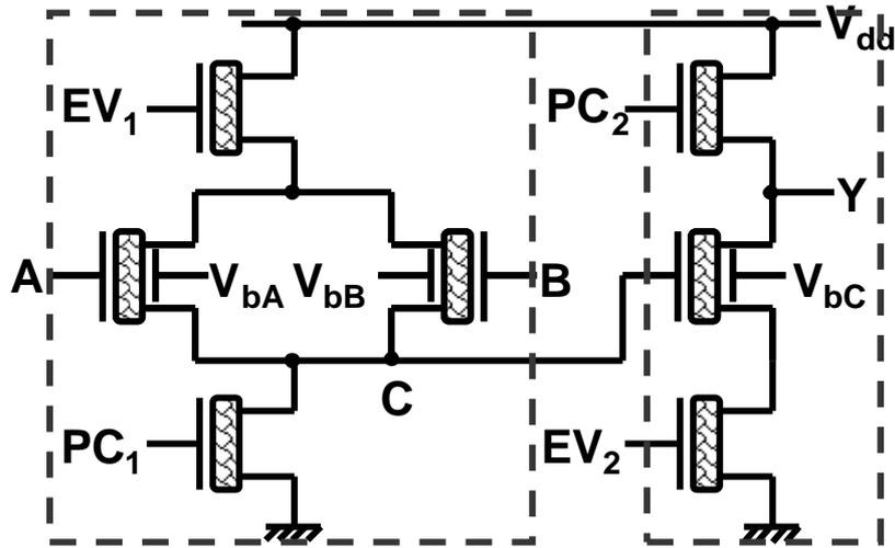
Fig. 3. Dynamically reconfigurable logic cell (DRLC\_7T) transistor-level schematic
