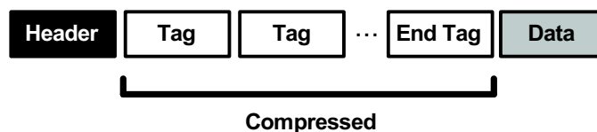
Figure 3. Appending data to an SWF file.
