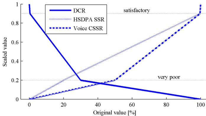
Fig. 1. Piecewise linear scaling of three radio performance KPIs.
