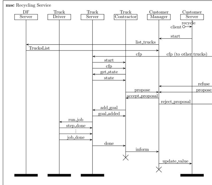
Fig. 1. Agent processes and message exchange in EcoTruck
