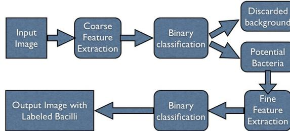
**Fig. 1.** The input original image passes through a front-end quick background subtraction system and drops most of background content. The filtered image (i.e., retained potential bacteria region) will be reanalyzed and reclassified with the purpose of improving the specificity of the whole system.
