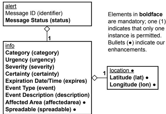
Figure 2. Enhanced CMAS CAP 1.2 alert message structure.
