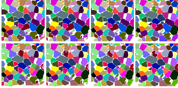
Fig. 7. First row, L^0 (at left) and its resampled versions at t \in \{0.33, 0.66, 1\} (at right). Second row, L^1 (at right) and its resampled versions at t \in \{0, 0.33, 0.66\} . Color points out voxels where nearest neighbor interpolation yields corresponding sets; white areas (at cell border) indicates that corresponding sets have to be searched further.
