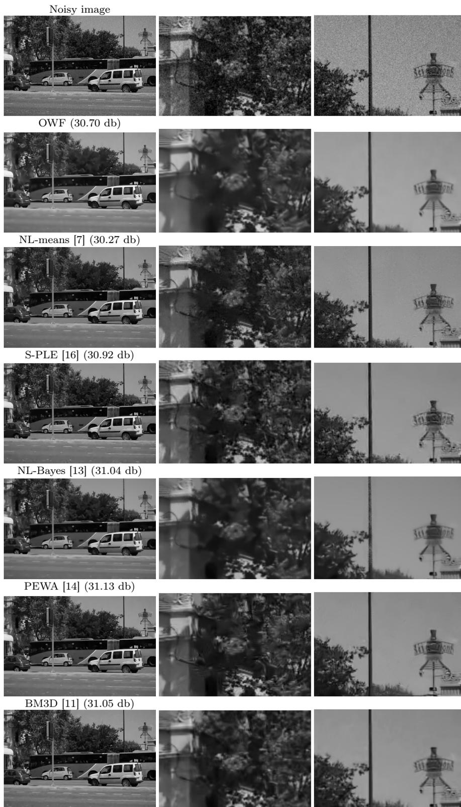
FIGURE 9 – Comparative results on the “traffic” image corrupted with WGN ( $\sigma = 20$ ). From top to bottom : noisy image, OWF, NL-means [7], S-PLF [16], NL-Bayes [13], PEWA [14], BM3D [11].
