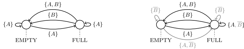
Fig. 1. Non-deterministic (left) vs. context-dependent (right) \text{LossyFIFO}_1 in Vereofy.
