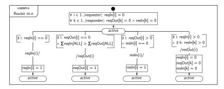
Fig. 4: UML notation for the EESM of Router m-n
