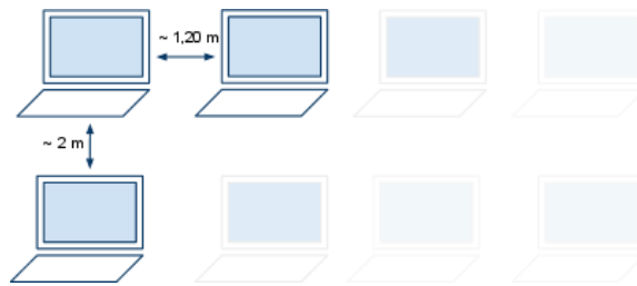
Fig.5 Default test setup
