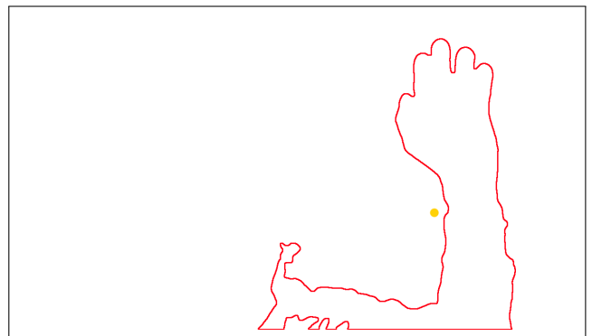
Figure 7. Detection of waving arm and hand in a video using OpenCV. The centroid of the contour is the yellow point left to the wrist.
