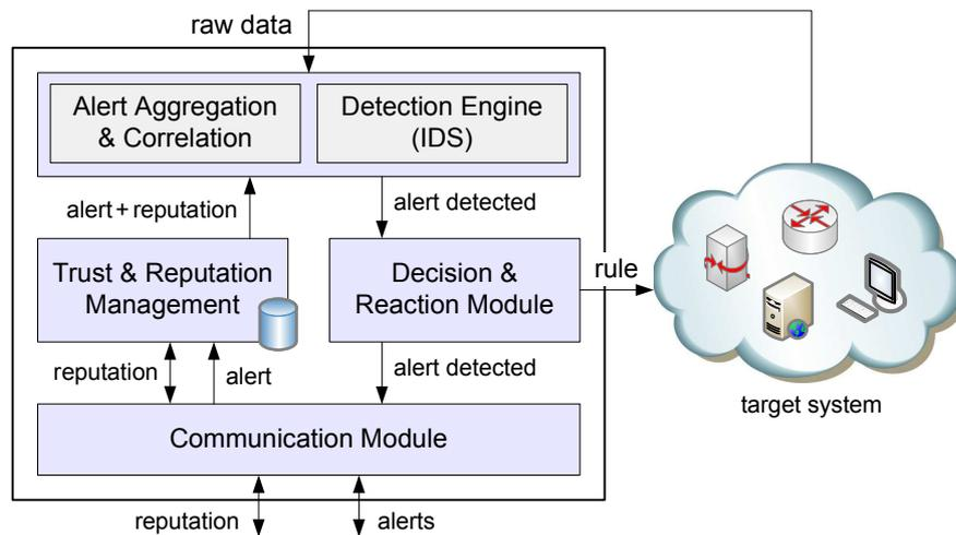
Fig. 2. Internal components deployed by an administration unit
