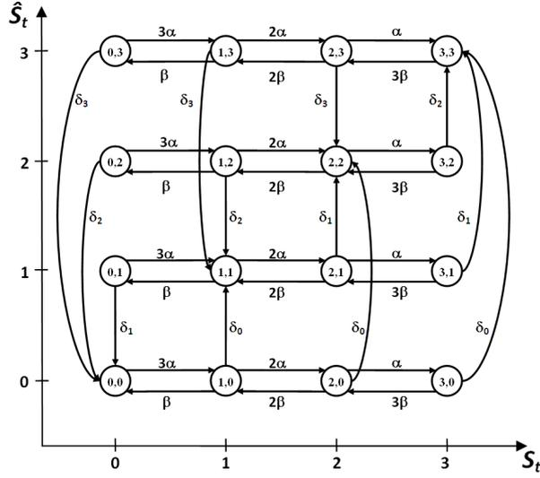
Fig. 1. CTMC of the  $\{S_t, \hat{S}_t\}$  process for  $M=3$ . The horizontal transitions describe the changes of environment state  $S_t$ . The vertical transitions describe the updates of the estimator  $\hat{S}_t$ .
