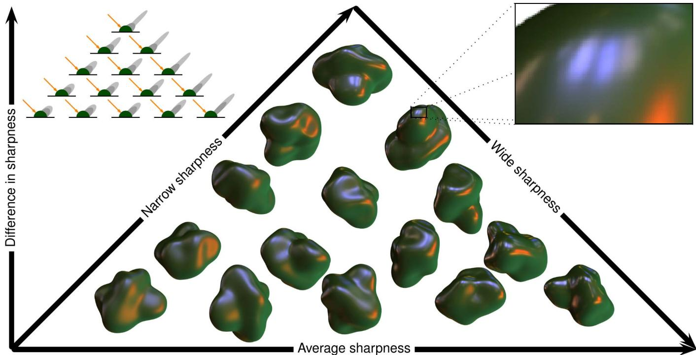
Figure 4. Triangular space of two-component glossy materials. Example target materials from the matching task are displayed at their correct location in the space. Only parameter values inside the triangle are valid according to our model (Equation 1). This limits the range of slider controls. Left inset: graphical representations of the corresponding BRDFs. Right inset: a zoom on a hazy reflection.
