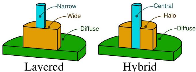
Figure 18. Schematic illustration of the layered decomposition based on the physical reflectances, and the hybrid decomposition that better predicts haziness.
